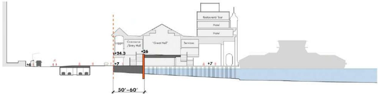
Figure 12: Flood defense alignment through the Battery Maritime Building
