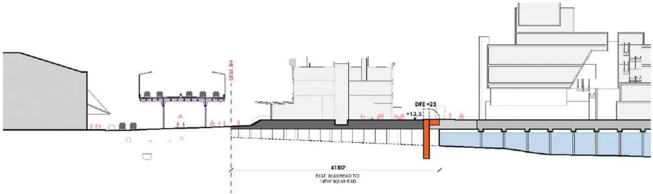
Figure 18: Flood defense alignment between the Tin Building and Pier 17 building
