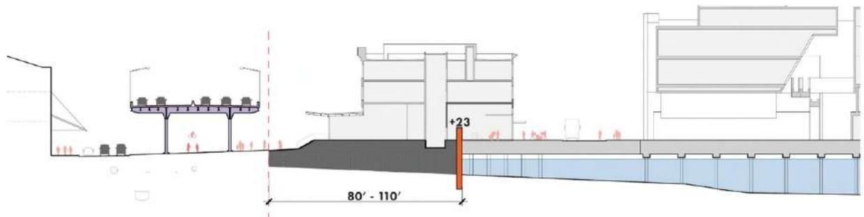
*Figure 17: Flood defense alignment through the Tin Building*
