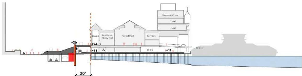
Figure 11: Flood defense alignment through the Battery Park Underpass
