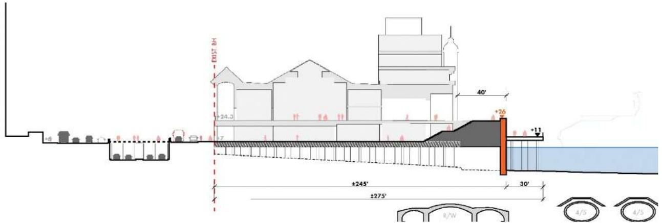
Figure 13: Flood defense alignment outboard of the Battery Maritime Building
