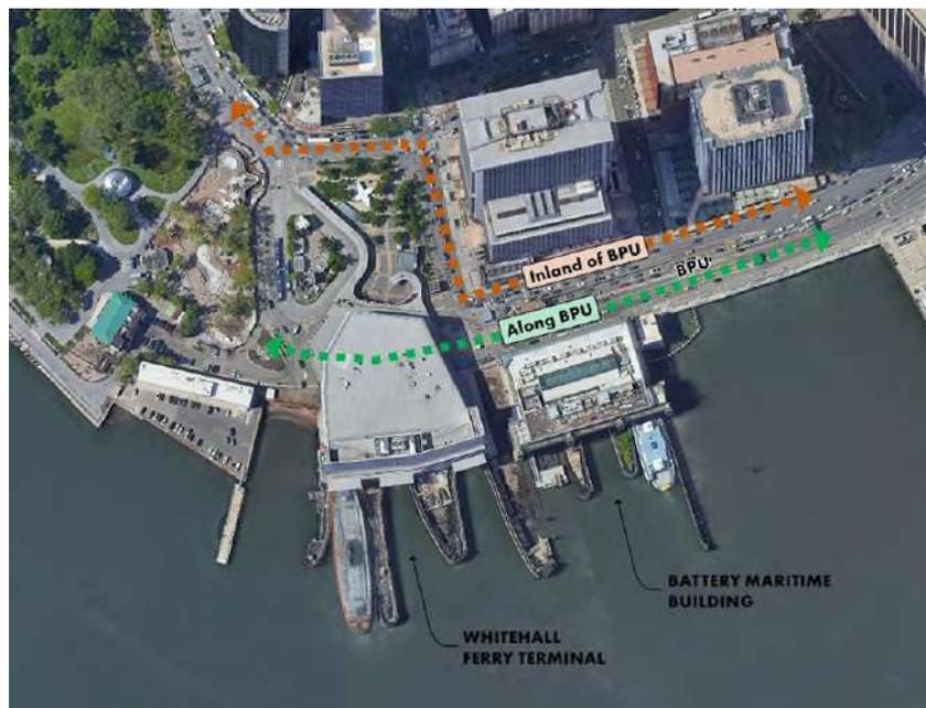
Figure 8: On-land alignment options between the southern tie-in and the Battery Maritime Building (Background source: Google Earth)
