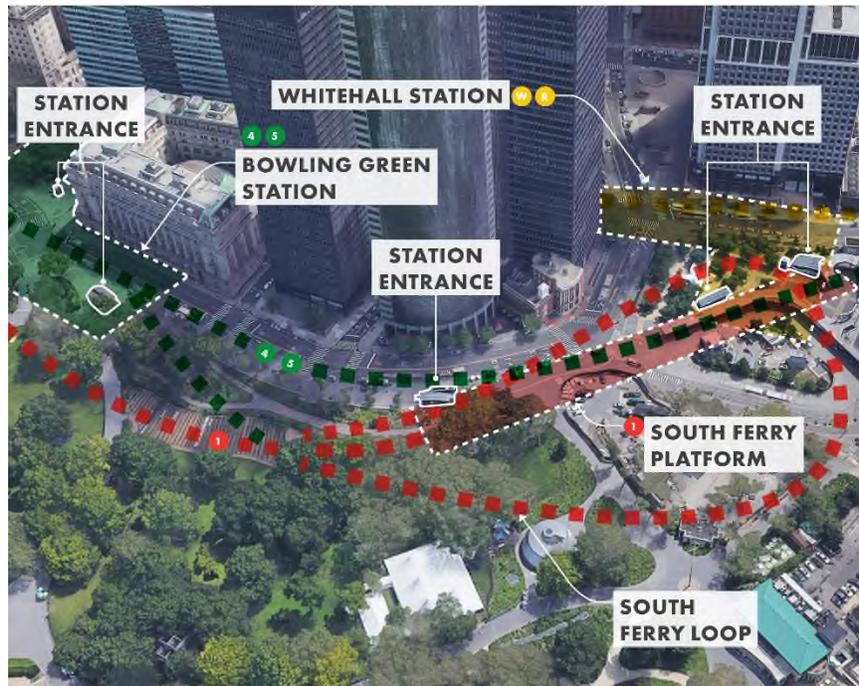
Figure 9: Overview of key subsurface infrastructure between the southern tie-in and Battery Maritime Building (Background source: Google Earth)
