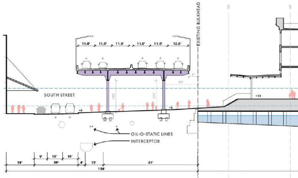
Figure 14: There is only about 6 feet of clearance between the FDR Drive viaduct and the existing bulkhead near the Tin Building.
