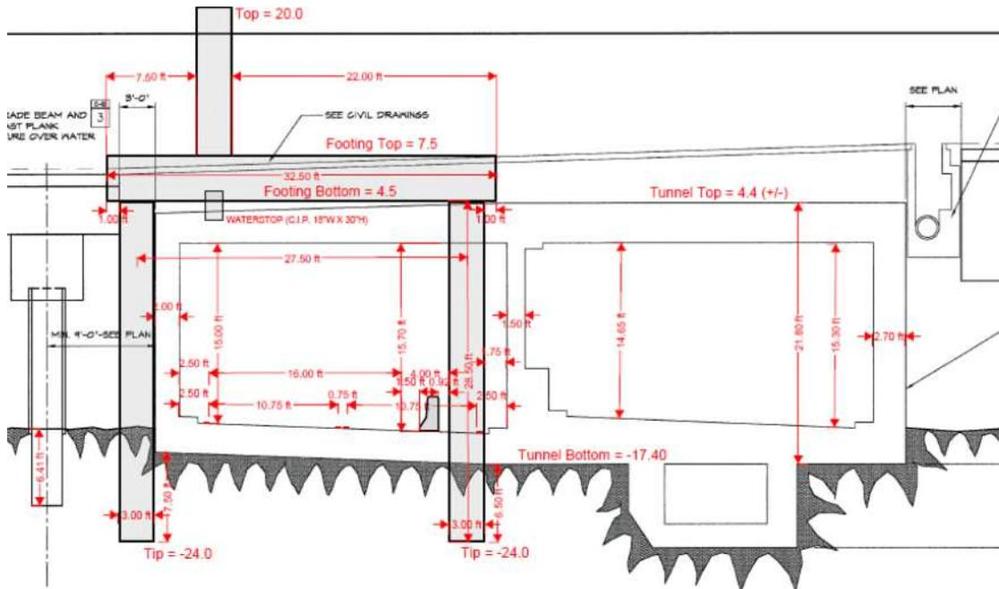
Figure 10: Schematic of potential modifications to the Battery Park Underpass needed to incorporate flood defense (representative cross section of the Battery Park Underpass; not intended for design)
