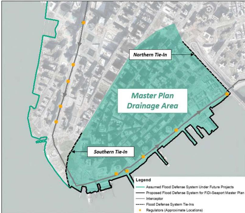
Figure 1. Study Area and Potential Alignment of Flood Defense Systems
