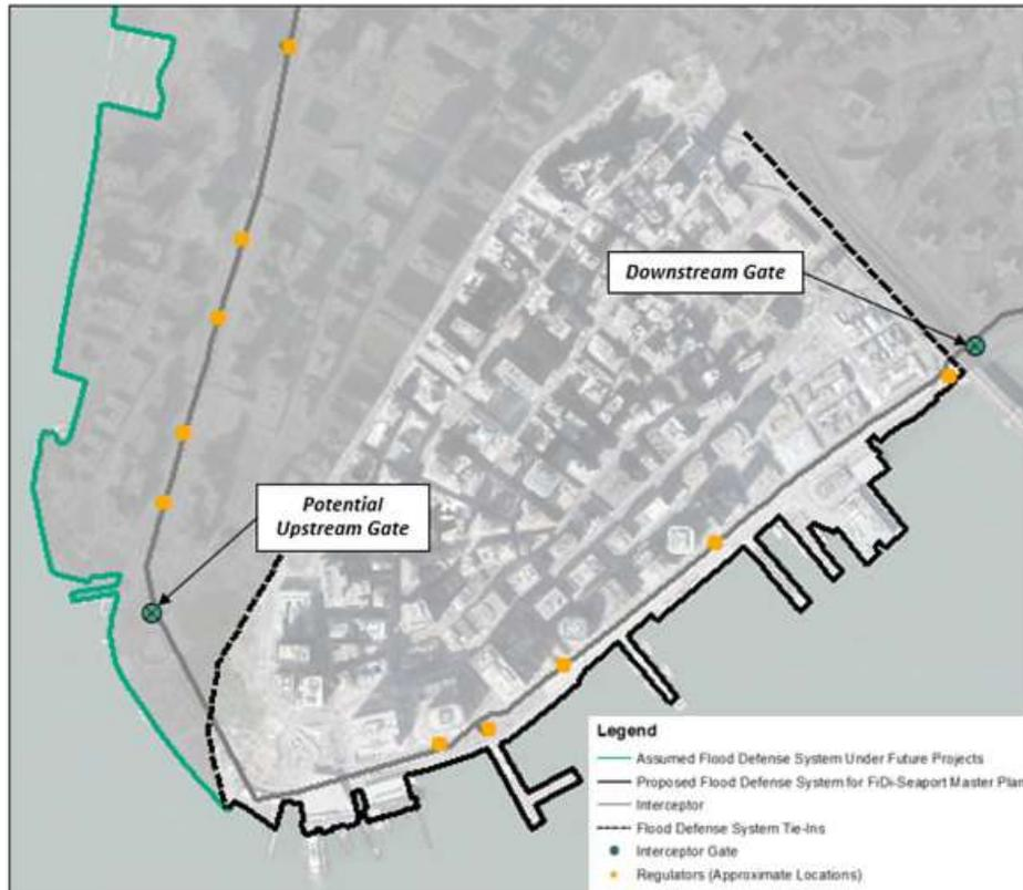
Figure 5. Locations of Modeled Downstream and Upstream Interceptor Gates
