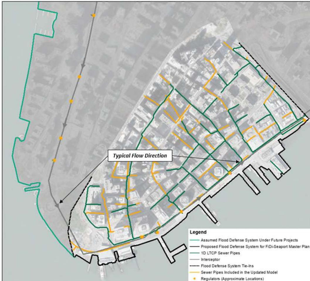
Figure 2. Sewer Network Buildout within Study Area
